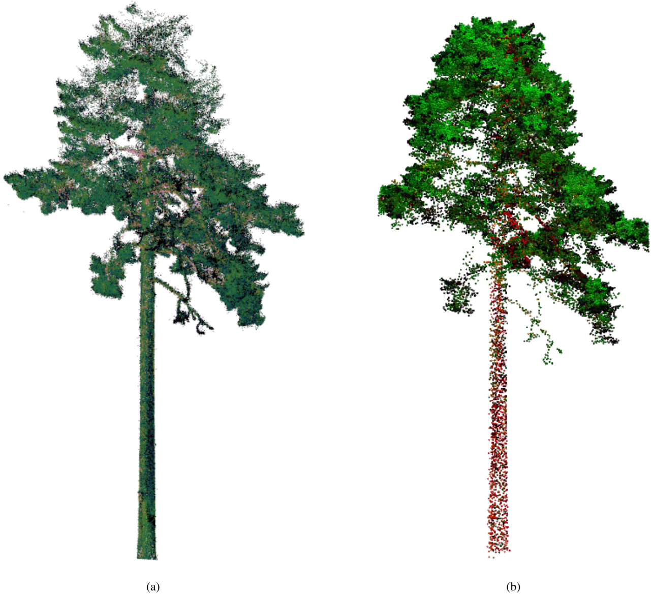
Figure 2: The same pine tree as captured by (a) the backpack mobile scanner, and (b) helicopter-ALS. The point counts of the segments are 399 239 and 94 586 respectively. The colouring of the points is purely for visualisation purposes.
