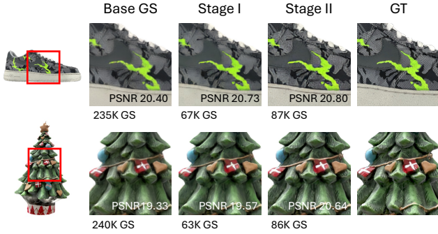
Figure 6. The effect of our two-stage pipeline on a local refinement task. Stage I achieves significant compression while maintaining visual fidelity. Stage II refines these compact GS, improving detail and overall quality based on the user’s input.
