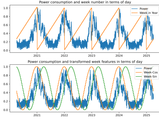
Fig. 2: Comparison between raw and transformed temporal features. (Top) Normalized power consumption plotted with the raw Week in Year feature, showing discontinuities at year boundaries. (Bottom) Same power series plotted with its cyclical encodings: Week-Cos and Week-Sin , which produce smooth and continuous representations across years.
