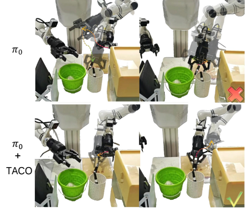
Figure 4 (Left) Efficiency improvement from KV cache optimization. For each number of action samples, we repeated the inference 50 times and reported the average inference time. (Right) A key moment from the Paper and Pen task, where the robot needs to pick up a marker. The base policy \pi_0 often falls into a suboptimal mode, causing the arm to swing back and forth and hesitate before grasping, which leads to task failure. In contrast, our method enables \pi_0 to completely avoid such oscillations and hesitation during grasping.
