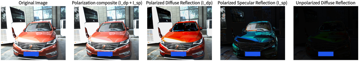
Fig. 3: Separation results of specular and diffuse components based on polarized images.
