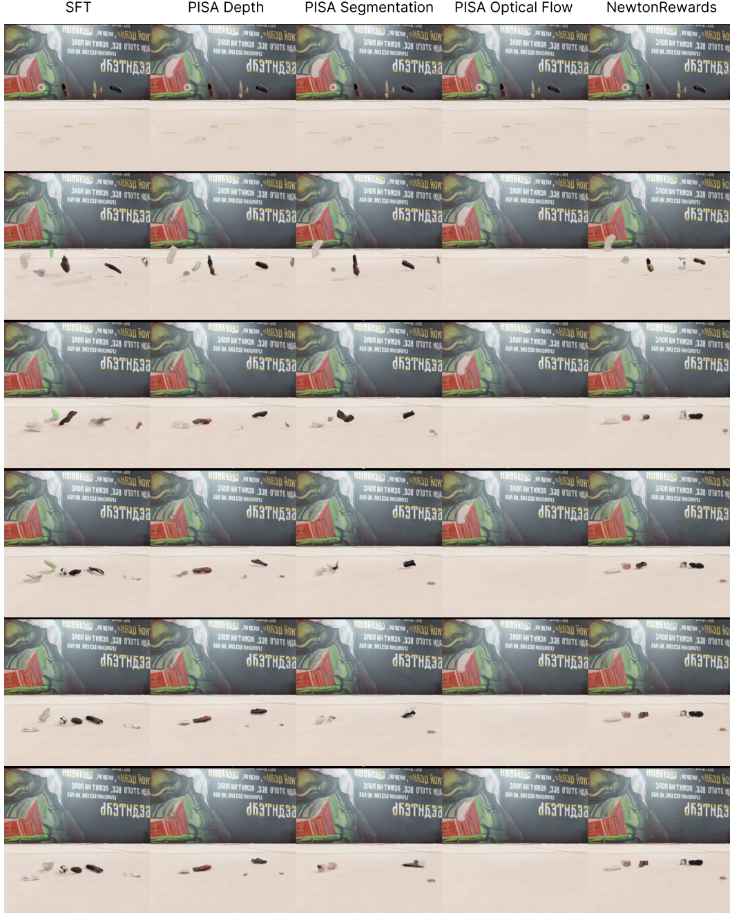
Figure 9. Qualitative comparison of post-training strategies on the NewtonBench-60K free fall scenario. Clear differences appear when examining the temporal evolution across frames (top→bottom). Under SFT and all PISA variants (Depth, Segmentation, Optical Flow), the objects frequently display inconsistent vertical acceleration and unstable trajectories sequence frames where items jitter, deviate laterally, or momentarily “hover”. PISA Optical Flow particularly exhibits frame-to-frame jitter and irregular descent. In contrast, NewtonRewards produces smooth, stable free-fall motion: objects drop along physically plausible vertical paths with consistent acceleration and minimal horizontal drift, closely matching true gravitational dynamics.
