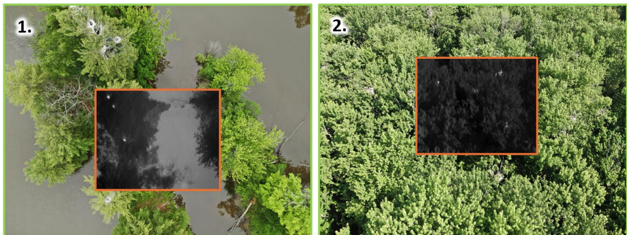
Figure 2 : Example of the field of view difference between corresponding visible image (green) and thermal image (orange) on a pair of nadir (1) and oblique (2) images.
