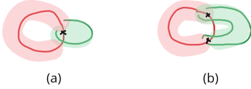
FIG. 6. Two loops of opposite types have to be braided more than once, because otherwise the correlation surfaces would not be correctly connected with each other. This observation is a criteria for checking the correctness of braided circuits. (a) incorrect connection of a red tube to the green sheet, because the tube would need to connect twice at the black braiding point; (b) the red tube can connect correctly to the green sheet, because now there two braiding points and each of these points is touched only once by the tube.
