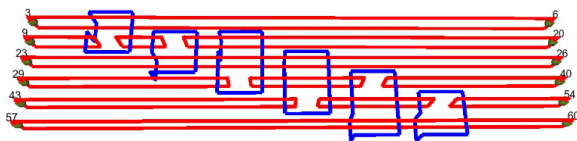
FIG. 3. Elements of braided circuits [4]: pairs of defects (here primal, red) form logical qubits and are braided with loops of the opposite type (here dual, blue) for performing CNOTs. The circuit herein does not include bridges.
