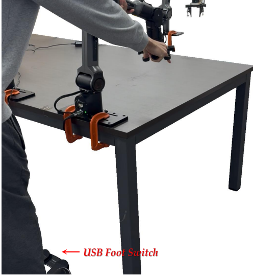
Fig. 7: Data collection based on homogeneous teleoperation hardware, where the suction cup is controlled by a foot-operated USB device.
