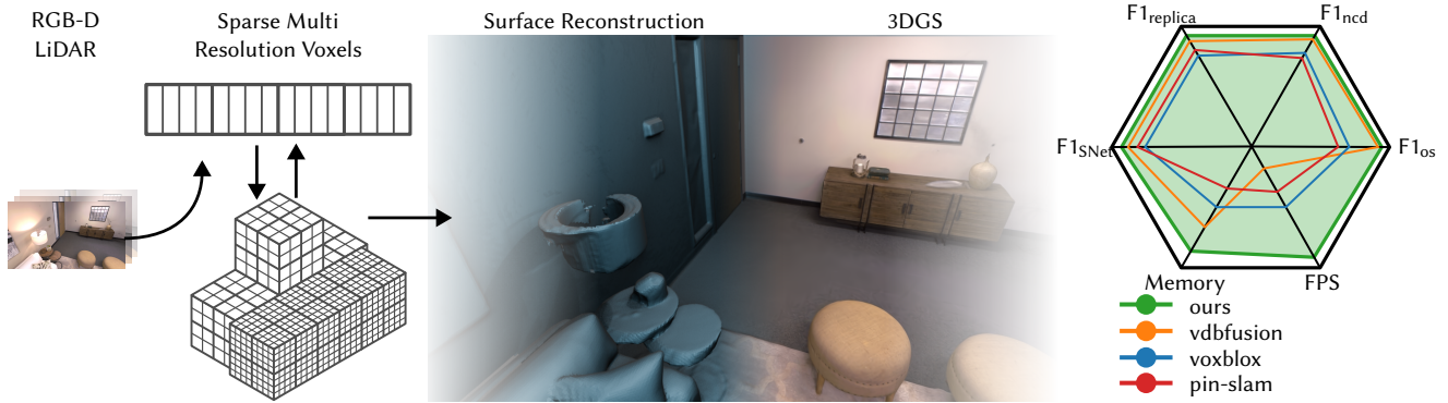
Fig. 1. Overview. Our pipeline for real-time 3D reconstruction and rendering. Left: Our variance-adaptive voxel grid dynamically adjusts resolution based on TSDF variance, enabling compact and accurate reconstructions from both RGB-D and unstructured 3D point clouds. The mesh output supports high-quality rendering via Gaussian Splatting, with adaptive splat control handled fully on the GPU. Right: Overview comparison reporting F-score across different datasets, memory efficiency, and FPS.
