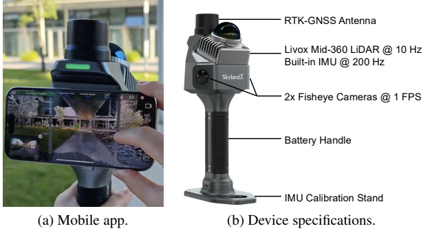
Figure 2. The MetaCam device. (a) SkylandX MetaCam Air used for data collection, equipped with a companion app for mobile capture. (b) Working frequency of each sensor.
