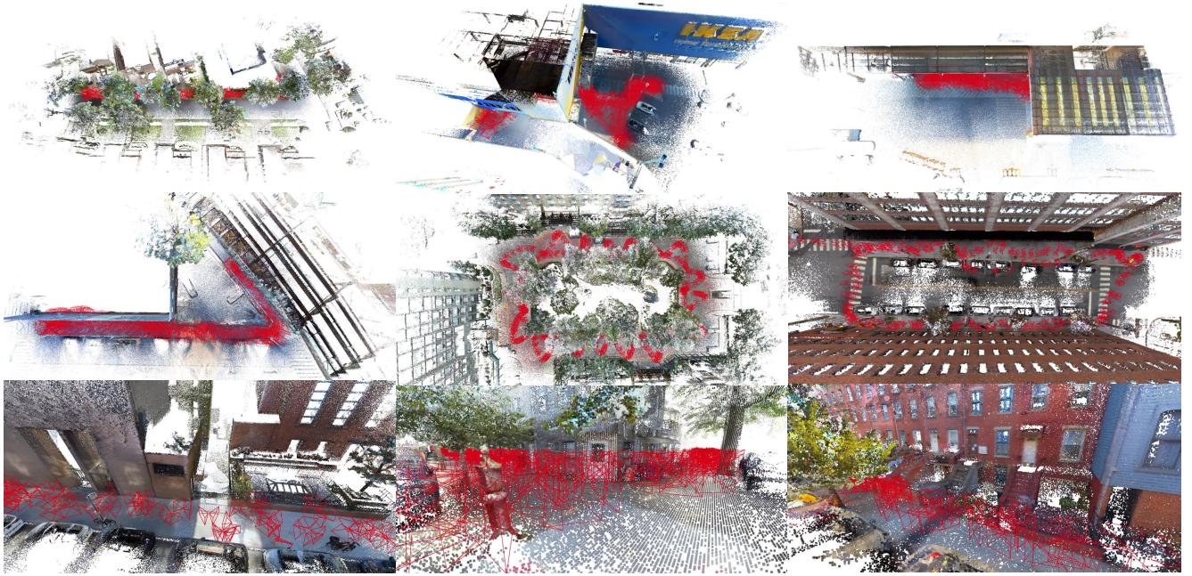
Figure II. Our 3D reconstruction from LIV-SLAM. The global colorized point cloud is downsampled for visualization cleanness.
