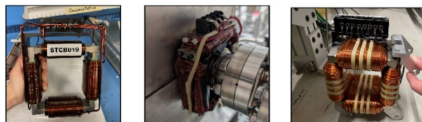
Figure 1: IPI magnet corrector elements, left to right: Dipole trim (Style #1), dipole trim (Style #2), multi-function corrector.
