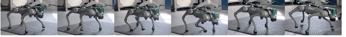
Fig. 2: Sequence illustrating the discovered walking gait on the Go2 quadruped.
