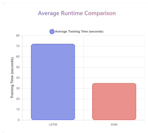
Figure 7: Average Runtime Comparison: KAN vs LSTM Training Times. KAN models demonstrate a significant 2.1 times speed advantage with average training times of 35.12 seconds compared to LSTM’s 75 seconds, showing superior computational efficiency for rapid prototyping and resource-constrained deployments.
