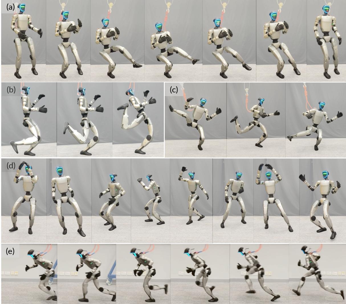
Fig. 1: Introducing AMS (Agility Meets Stability), one single policy that performs diverse motions with stability and agility simultaneously on a humanoid robot. The robot can execute challenging balance motions such as (a) Ip Man’s Squat, a Kung Fu-style single-leg squat, unseen during training (zero-shot); (b) single-leg balance stances which humans find hard to perform; (c) balanced stretching; as well as expressive motions and high-mobility movements with precise control, such as (d) dancing and (e) running. More examples are provided in the appended video.
