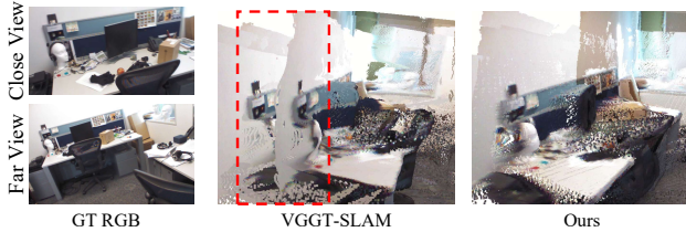
Figure 4. Qualitative Comparison of Reconstructed Point Clouds on office. Left: RGB images from different views. Middle: VGGT-SLAM. Right: SING3R-SLAM (Ours). Our approach accurately aligns the wall and table across views, whereas VGGT-SLAM produces misaligned and overlapping geometry.
