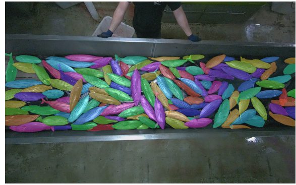
Figure 2. Manually annotated image. This image contains a masks for each fish on the conveyor belt that is visible from the point of view of the camera. This frame belongs to a monospecific SKJ sample. It was used during the training of the models.
