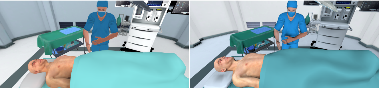
Figure 6: Enhanced Realism with GA-Powered Neural Rendering: (Left) Standard Unity engine lighting on a dynamic character. (Right) The same scene rendered with our "NeuralGASh" pipeline, which achieves superior, dynamic lighting and shadow fidelity without pre-computation [3].
