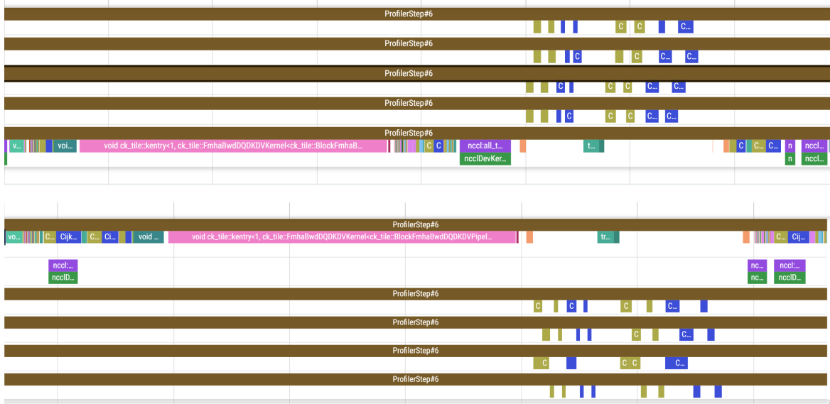
Figure 10: DeepSeek-V2-Lite pre-training backward-pass layer execution (Top) regular connectivity (Bottom) FarSkip-Collective. The backward-pass operator execution order is “hijacked” from the default torch.autograd Sequence Number ordering to re-order operations for overlap. In particular, routed-expert backward computation launches immediately after the finished synchronization point of the Combine all-to-all backwards gradient and the Dispatch gradient launches before the gradient of the first part of attention ( q, k, v calculation) to allow for overlapping with it before synchronization.
