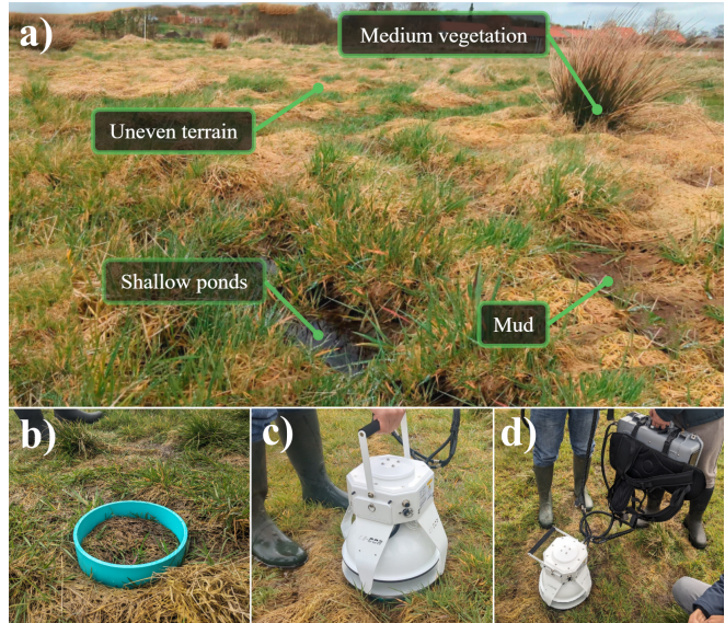
Fig. 1: Field sampling workflow in Danish wetlands. (a) Overview of the sampling area. (b) A PVC collar is pushed and fixed into the ground. (c) A chamber is seated on the collar for gas collection. (d) Two portable gas analyzers carried by the researchers complete the GHG readings.
