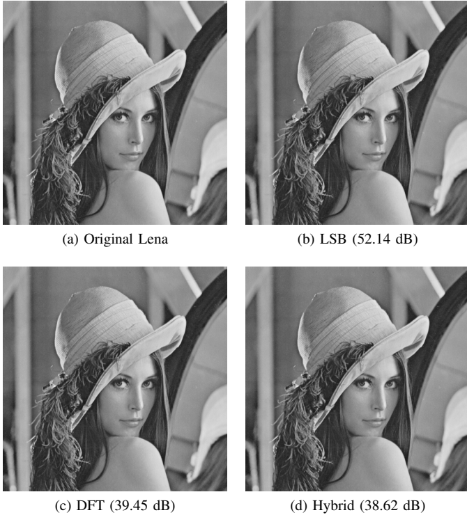
Fig. 2: Visual comparison of watermarked 'Lena' images (Original vs LSB, DFT, Hybrid).
