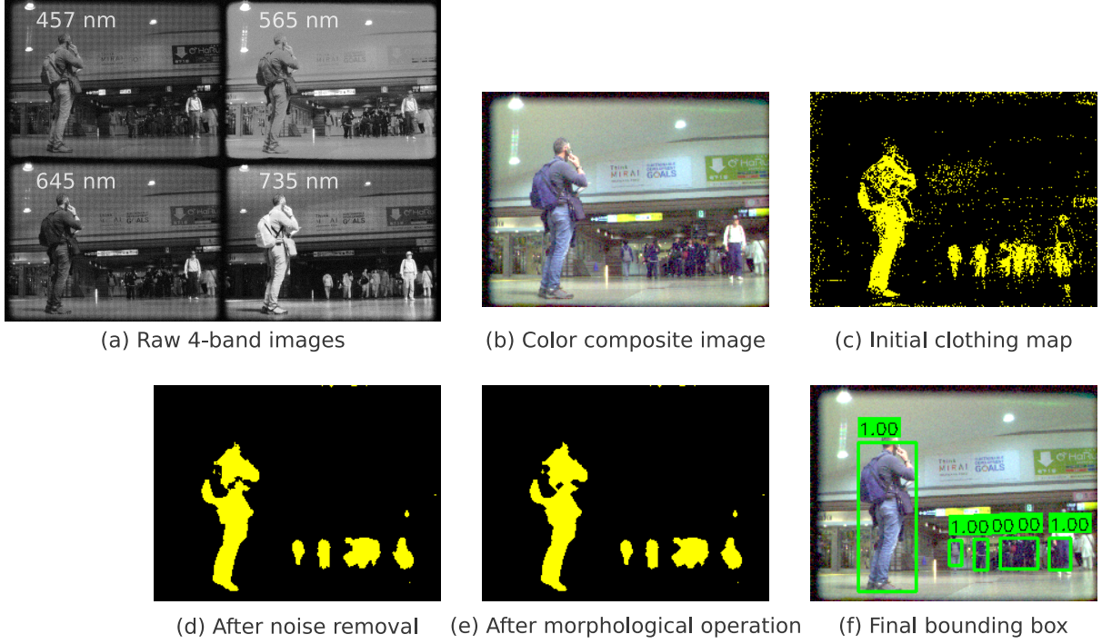
Figure 5: Example of entire processing sequence from 4-band image acquisition to final bounding box generation. (a) Raw 4-band images captured by camera. (b) Color composite image synthesized for easy viewing. The band assignments are R=645, G=565, and B=457 nm. (c) Initial map of pixels classified as "clothing" by MLP. (d) Map after noise removal. (e) Map after morphological operations are applied to define continuous regions. (f) Final bounding box calculated for defined clothing region.
