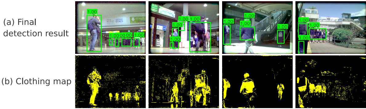
Figure S-3: Qualitative results of HitoMi-Cam in the General Scene. (a) Examples of final detection results. (b) The corresponding examples of intermediate clothing maps.
