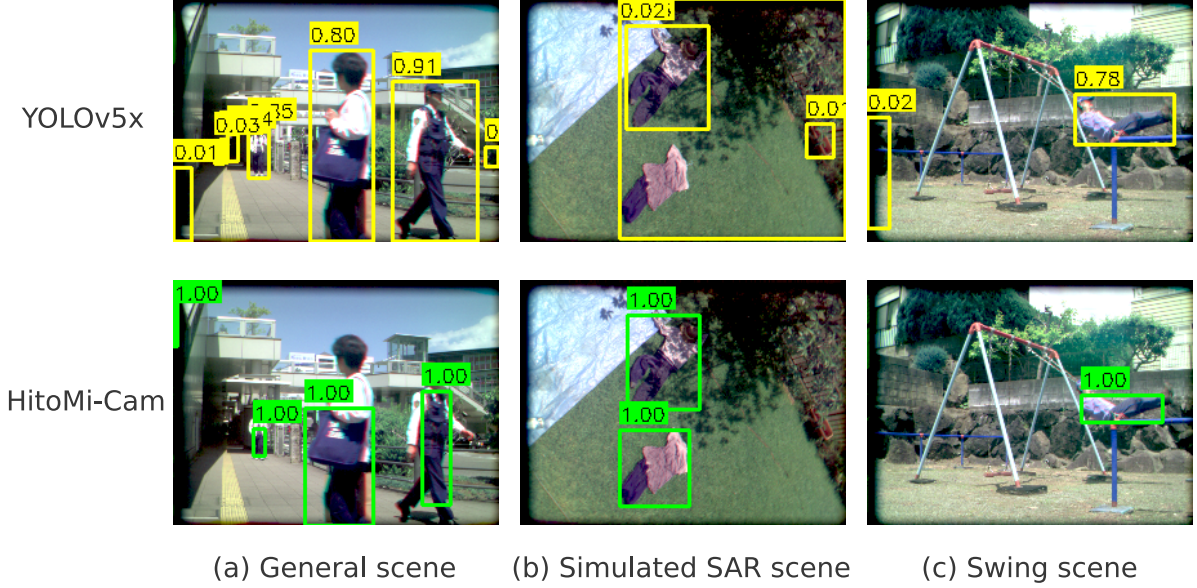
Figure 7: Comparison of representative frames and detection results from the three datasets. Yellow indicates results from the comparison method (YOLOv5x), and green indicates HitoMi-Cam results. (a) In the case of General Scene, the CNN (yellow) shows high accuracy, while HitoMi-Cam (green) detects only the clothing area, generating a smaller rectangle. (b) In the case of Simulated SAR Scene, detection by the CNN (yellow) fails because the target does not have a human shape, but HitoMi-Cam (green) captures the material characteristics and detects the ground truth. (c) In the Swing Scene, the CNN’s (yellow) detection becomes unstable for atypical postures, while the shape-agnostic HitoMi-Cam (green) continues to track the target.
