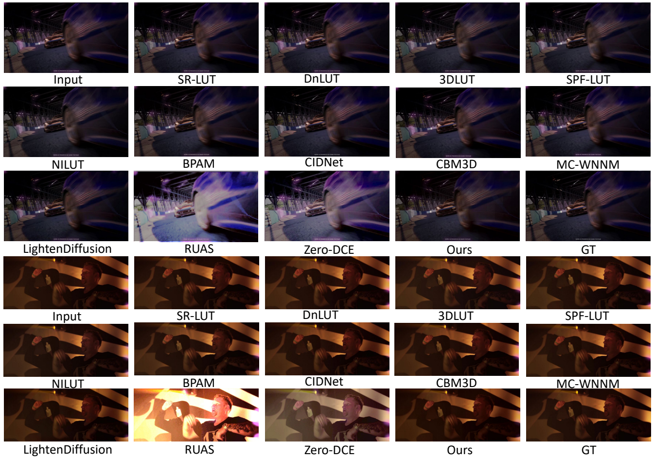
Figure 13: Visual comparison of all methods on a challenging night scene from the PFSD dataset. Our method effectively removes the purple flare around the lights while preserving details in the dark areas.
