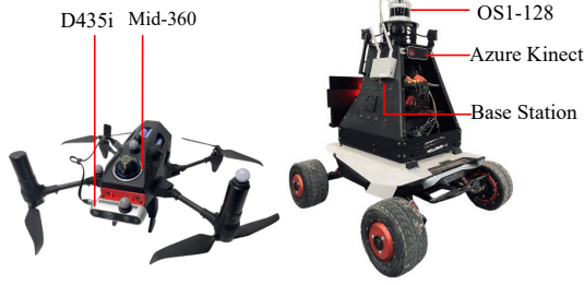
Fig. 3. Hardware Configurations of UAV and UGV.
