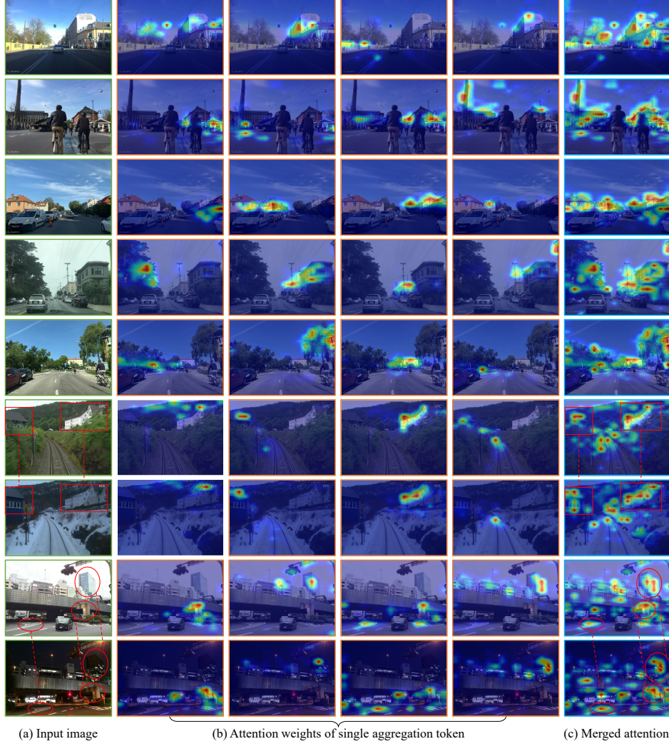
Figure 5: The visualization of the attention weights of our agg tokens to patch tokens. The first column (a) represents the input images. The middle 2-5 columns (b) separately display the attention weights of a single agg token to all patch tokens (reshaped to restore spatial position), meaning each image shows the attention of only one agg token. The last column (c) shows the merged attention of all 8 agg tokens. The first five examples ( i.e. , five rows) show five different places, with buildings, vegetation, and dynamic interference. While different agg tokens attend to distinct regions (or objects) in the images, they consistently focus on stable and discriminative areas ( e.g. , buildings and vegetation), while largely ignoring variable elements ( e.g. , cars). The sixth and seventh examples show two images taken at the same place in different seasons. Our agg tokens can consistently focus on buildings (and some discriminative regions where the terrain and railroad tracks change). The last two examples demonstrate that agg tokens can consistently focus on buildings and landmarks even after undergoing severe lighting changes.
