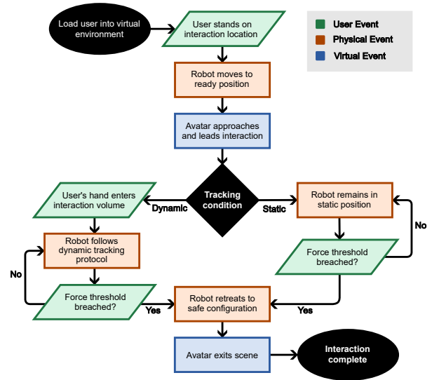
Fig. 3. Flowchart depicting the consistent sequencing of user and system actions for all interactions presented in this work: object handover, fist bump, and high five.
