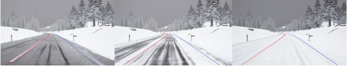
Fig. 2: Different snow levels incorporated in the SnowyLane dataset. Low snow (left), medium snow (mid), and high snow (right)
