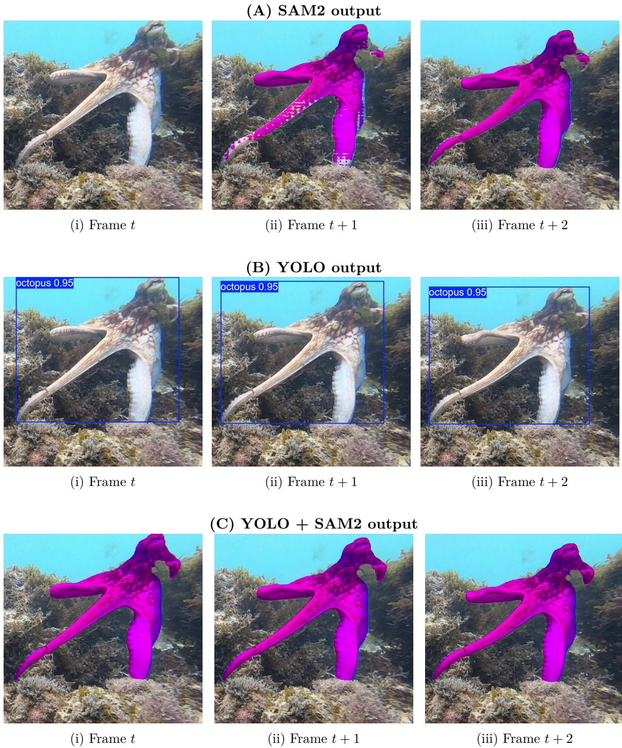
Figure 3: Example of three consecutive frames on how to use YOLO in conjunction with SAM2. (A) SAM2 initially fails to recognize the octopus, producing a noisy, speckled segmentation mask before eventually generating a coherent result; (B) The specialized YOLO model successfully detects the octopus from the very first frame; (C) When the YOLO detections are used as prompts for SAM2, accurate segmentation masks are produced from the beginning of the sequence. Thus, we infer that the target object was not abruptly lost during processing; any degradation likely occurred gradually or along the segmentation boundaries.
