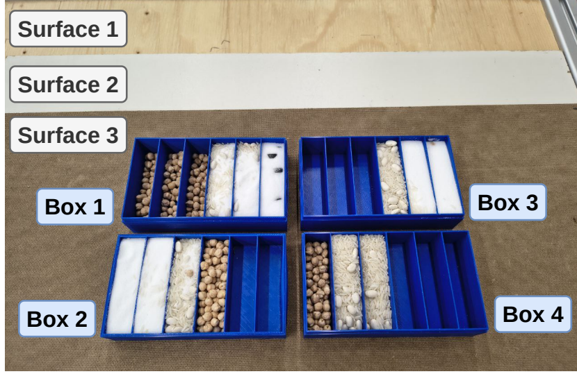
Figure 3: Context configurations used for real-world evaluation of the pushing task with center of mass variation, obtained by combining 3 surface materials 4 box variants. The surface materials differ in their friction coefficients, while the boxes vary in both mass and mass distribution, achieved by redistributing the filling material using internal separators.
