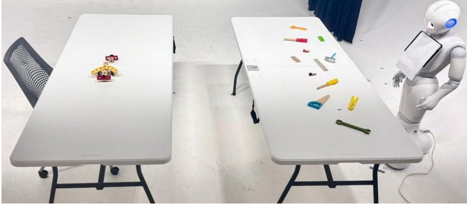
Fig. 4 Experiment setup. Left Task Table : Two pre-assembled parts for participants to start building the airplane model. Participants sat approximately 3.3 meters away so they could see the indicators in full. Right Robot Table : Objects within the robot's reach and needed to finish assembly.
