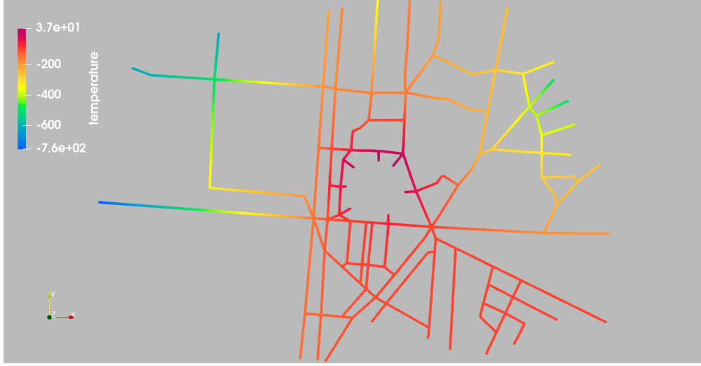
Figure 3: Optimized potential field u for the stadium network. Hotter colors (red–yellow) mark entrances or high-pressure zones; cooler tones (blue–green) mark exits and dissipative corridors. The reference potential was fixed at node 113 ( u_{113} = 10 ).
