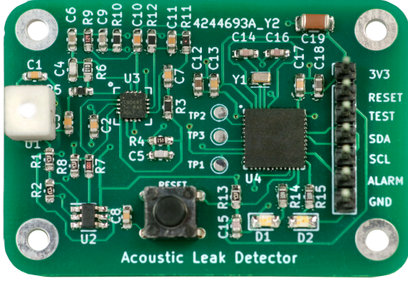
Fig. 1. The sensor PCB measures 48 mm x 33 mm. A surface mount MEMS microphone is enclosed by a rectangular chamber to form a Helmholtz resonator (far left). The 7-pin connection header is used for programming the MCU, I 2 C communication, and 3V3 dc power.
