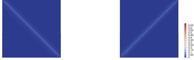
FIGURE 5. (U_x, U_y) = (0.5, -0.45) : loading configuration with multiple solutions. Phase fields for mesh \mathcal{T}_A (left) and mesh \mathcal{T}_B (left) at (U_x, U_y) = (0.01, 0.009) . In both cases it is localized on a strip of width \epsilon_h = 0.025 .
