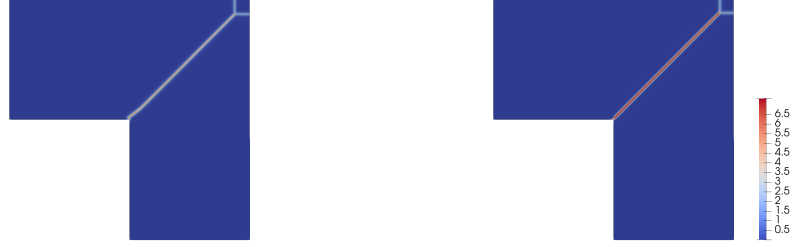
FIGURE 10. Strain for mesh \mathcal{T}_A (left) and mesh \mathcal{T}_B (left) at t = 39 . In both cases it is localized on a strip of width h = 0.005 .
