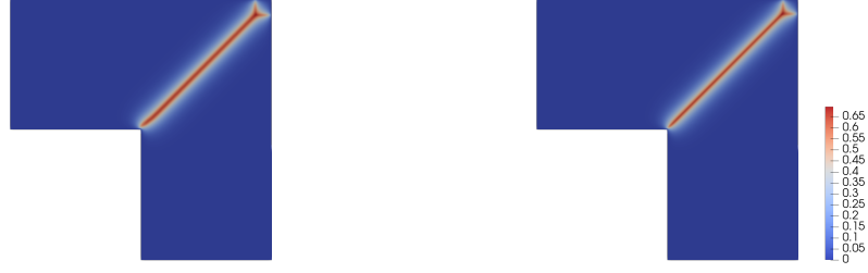
FIGURE 9. Phase fields for mesh \mathcal{T}_A (left) and mesh \mathcal{T}_B (left) at t = 39 . In both cases it is localized on a strip of width \epsilon_h = 0.025 .
