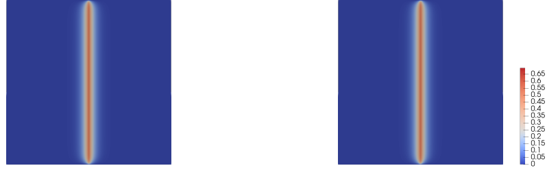
FIGURE 6. (U_x, U_y) = (1, 0.5) : loading configuration with unique solution. Phase fields for mesh \mathcal{T}_A (left) and mesh \mathcal{T}_B (left) at (U_x, U_y) = (0.017, 0.0085) . In both cases it is localized on a strip of width \epsilon_h = 0.025 .
