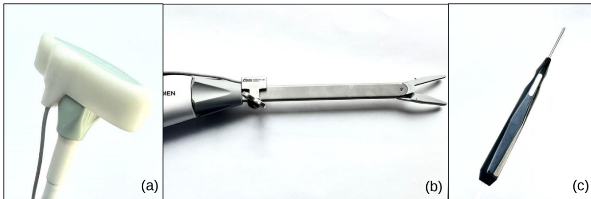
Figure 1: EM tracked surgical instruments used in this study: (a) intraoperative ultrasound transducer, (b) vessel sealer, (c) surgical pointer
