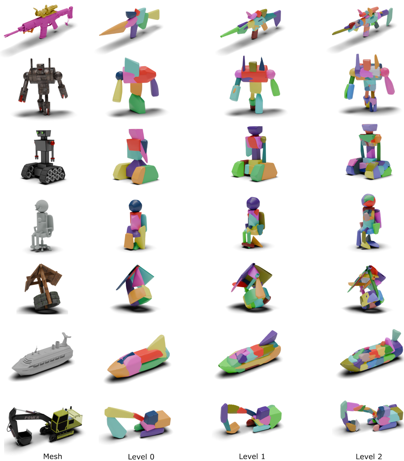
Figure 11. Hierarchical decomposition results on Objaverse dataset [9]. First column indicates the ground truth mesh from which points are sampled for our network input. Next 3 columns indicate hierarchical decomposition at multiple granularities predicted by our model.
