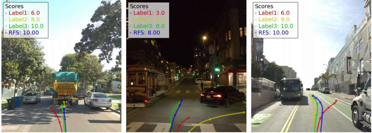
(a) The model predicted future trajectory (blue) aligns well with one of the rater specified trajectories. The corresponding flat scores are assigned as the predictions fall within the trust region.
