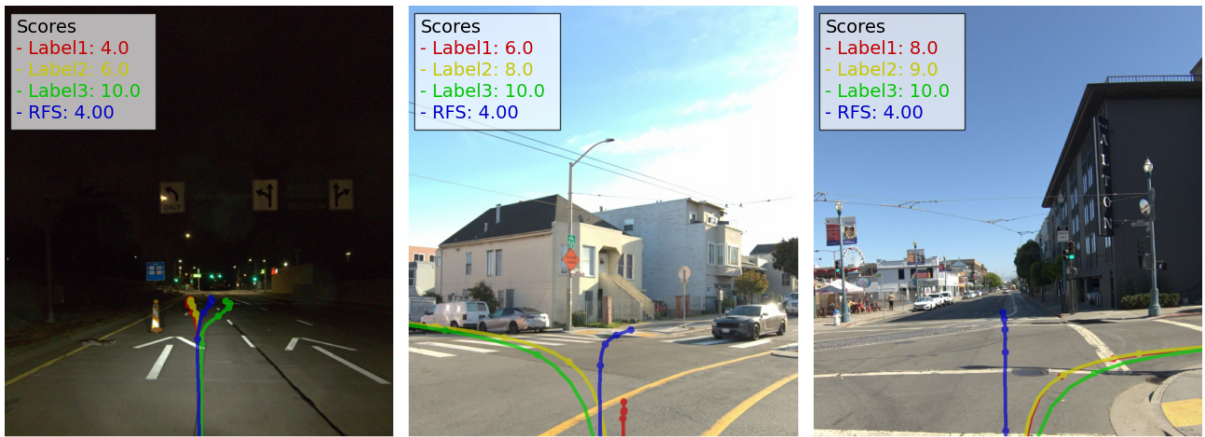
(c) Floored scores (RFS=4) are assigned because predictions are far from any of the rater-specified trajectories.
