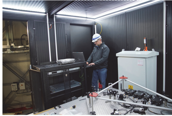
Figure 7. The PLACID cabinet infrastructure – a PC server unit (1U), a KVM unit (1U) and an interface box (2U) - was installed on the Nasmyth server rack on July 3rd, 2025. Note that the depicted cabinet will be later replaced by a liquid-cooled unit over the fall of 2025, to mitigate turbulence inside the Nasmyth enclosure.
