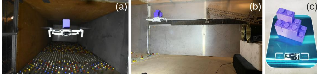
Fig. 4. Drone measurements in the wind tunnel. (a) Photograph of the drone hovering in the wind tunnel. The wind is always coming from one side of the drone; in this photo, it's coming from the back. The colored cubes at the bottom are used to create a stronger boundary layer from the bottom, mimicking, to some extent, the stronger turbulence in the atmospheric boundary layer environment below the drone. (b) The drone is positioned against the Tx and Rx radar antennas. The wind is from left (upstream) to right (downstream). (c) Calibration of payload weight.
