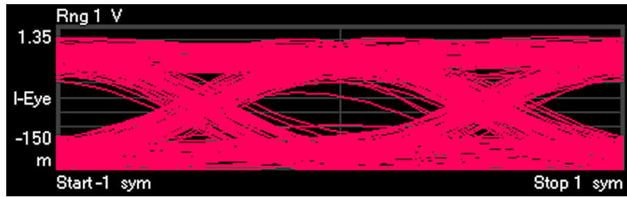
Fig. 5. Eye diagrams of the 2.97-Gb/s OOK signal. The corresponding Q-factor and BER are 5.32 and 5.20 \times 10^{-8} , respectively. Both values satisfy the HD-FEC limit (Q-factor = 2.67, BER = 3.8 \times 10^{-3} ).
