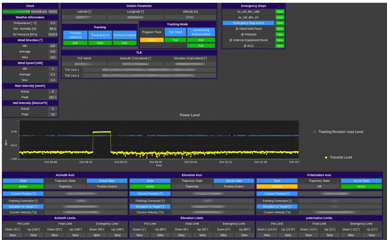
Figure 5: Example operator-created HMI fed by live satellite and ground telemetry data
