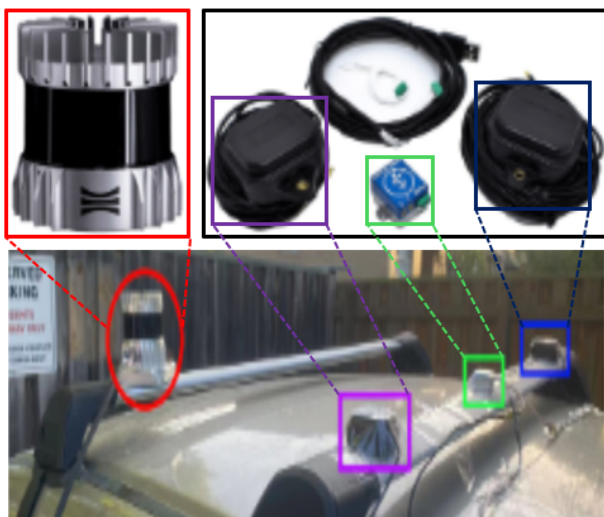
FIGURE 3: Sensor rig and installation. The system comprises an Ouster OS1-128 LiDAR, a dual-antenna RTK GNSS with MEMS IMU, and a logging unit mounted on a reinforced roof plate with a measured antenna baseline.
