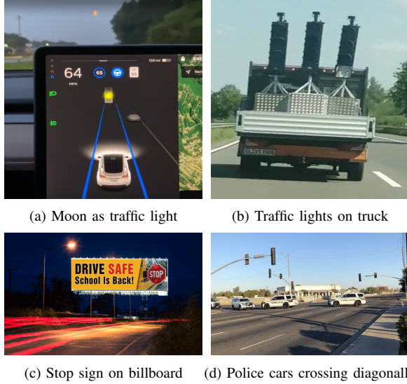
Fig. 2. Examples of semantic anomalies in autonomous driving scenarios. These real-world cases demonstrate contextually unusual situations where individually recognizable objects combine to create potentially unsafe or confusing scenarios for autonomous systems.
