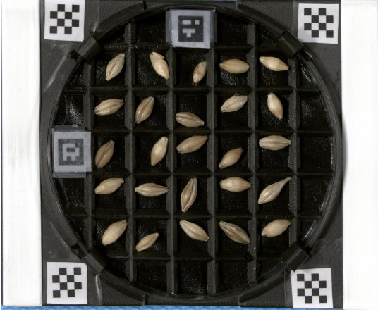
(i) The image resulting from size-correction of the colorized version of Figure 6h using bilinear interpolation with a factor based on the ratio between the height and width of the chessboard squares.
