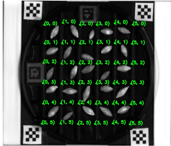
(d) A grayscale visualization of the HSI image corresponding to the RGB image in Figure 4c. The placement of the grid is derived based on an affine transformation between the centers of the 4 chessboards in Figure 4c and those in this image.
