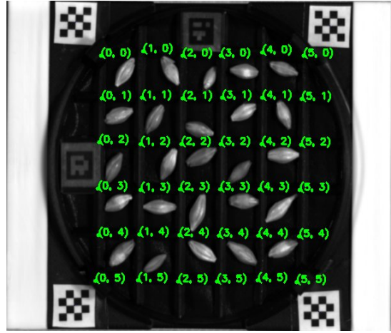
(j) The Petri dish from Figure 7a. Using the RANSAC algorithm (Fischler and Bolles 1981), an affine transformation matrix from Figure 6j to Figure 7i is computed based on the four chessboard centers. This affine transformation matrix is then used to move the grid from Figure 6j to Figure 7i without having to redetect the grid.
