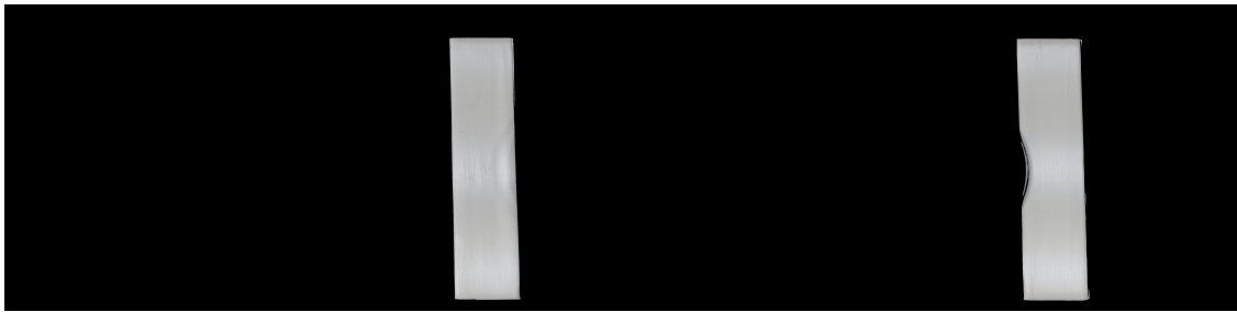
(e) Applying Figure 5d as a binary mask to Figure 5a to extract the white references.
