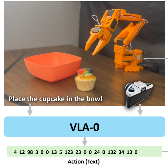
Fig. 1: Schematic representation of VLA-0. VLA-0 converts a VLM into a VLA by prompting the VLM to predict action as text. This strategy is surprisingly effective and achieves state-of-the-art results akin to alternatives.
