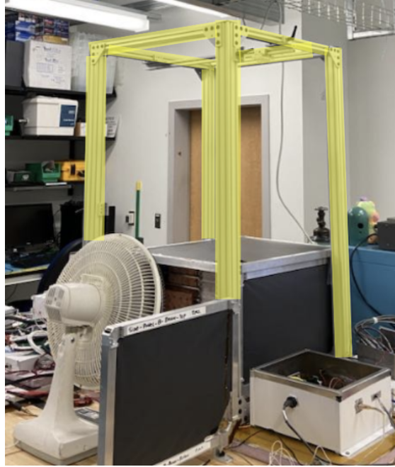
Figure 9: Calibration structure (highlighted) placed around the full ComPair instrument. This structure was used to hold radioactive sources in precise locations during calibrations. The main instrument stack is surrounded by the ACD (in black). One of the ACD panels is open, allowing a fan to cool the instrument to prevent overheating during operation. The ACD electronics box (white box) sits beside the ACD.
