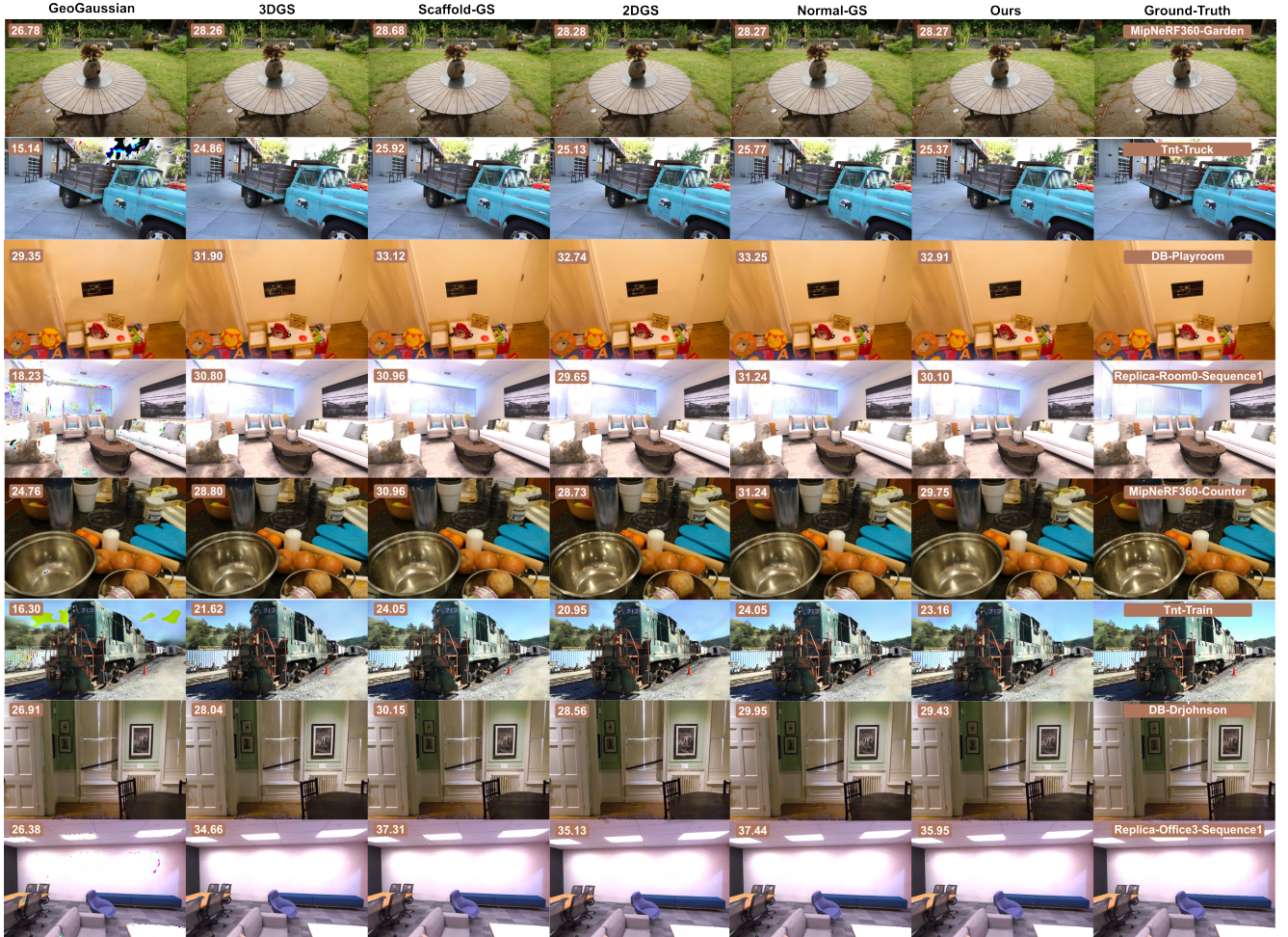
Figure 8. Qualitative comparison results on NVS demonstrate that our RGB rendering achieves better performance in certain scenarios. The top-left corner of the image displays the PSNR value computed against the ground truth image.
