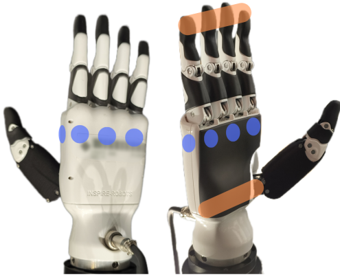
Fig. 3: The force application regions for the perception experiment. The blue regions correspond to Level 2, comprising eight distinct areas, while the orange regions represent Level 3, consisting of two areas.
