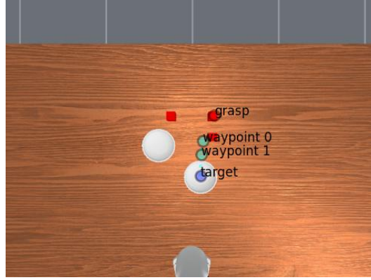
Figure 96: Keypoint generation using MOKA. As shown in the figure, MOKA generates ‘grasp’, ‘waypoint’, and ‘target’ keypoints for each task, and translates them into motion trajectories.
