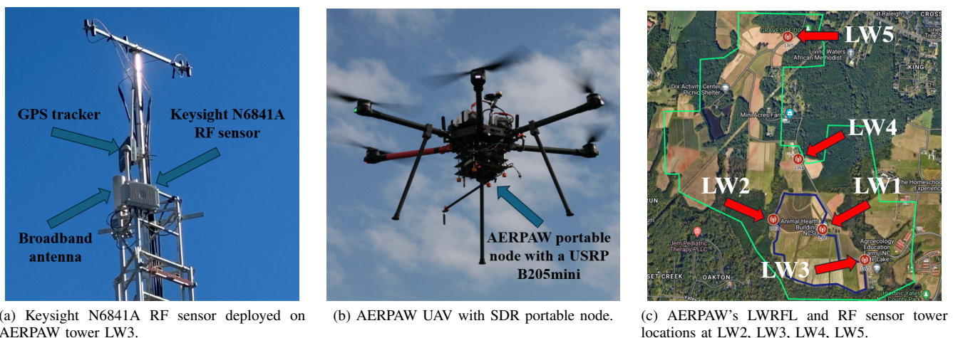
Fig. 23: Overview of the AERPAW testbed showing the RF sensor, UAV node, and LWRFL site layout [48].
