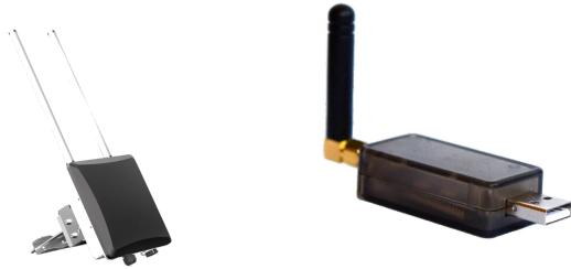
Fig. 17: LoRaWAN gateway and a USB-compliant programmable LoRa device, used in the AERPAW system for mobile LoRa experiments.
