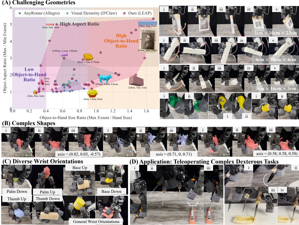
Figure 1: We introduce DexNDM , a sim-to-real approach that enables unprecedented in-hand rotation in the real world. We master a wide object distribution, including (A) challenging geometries and (B) complex shapes, across (C) rich wrist orientations. (D) A teleoperation application. Videos in website .
